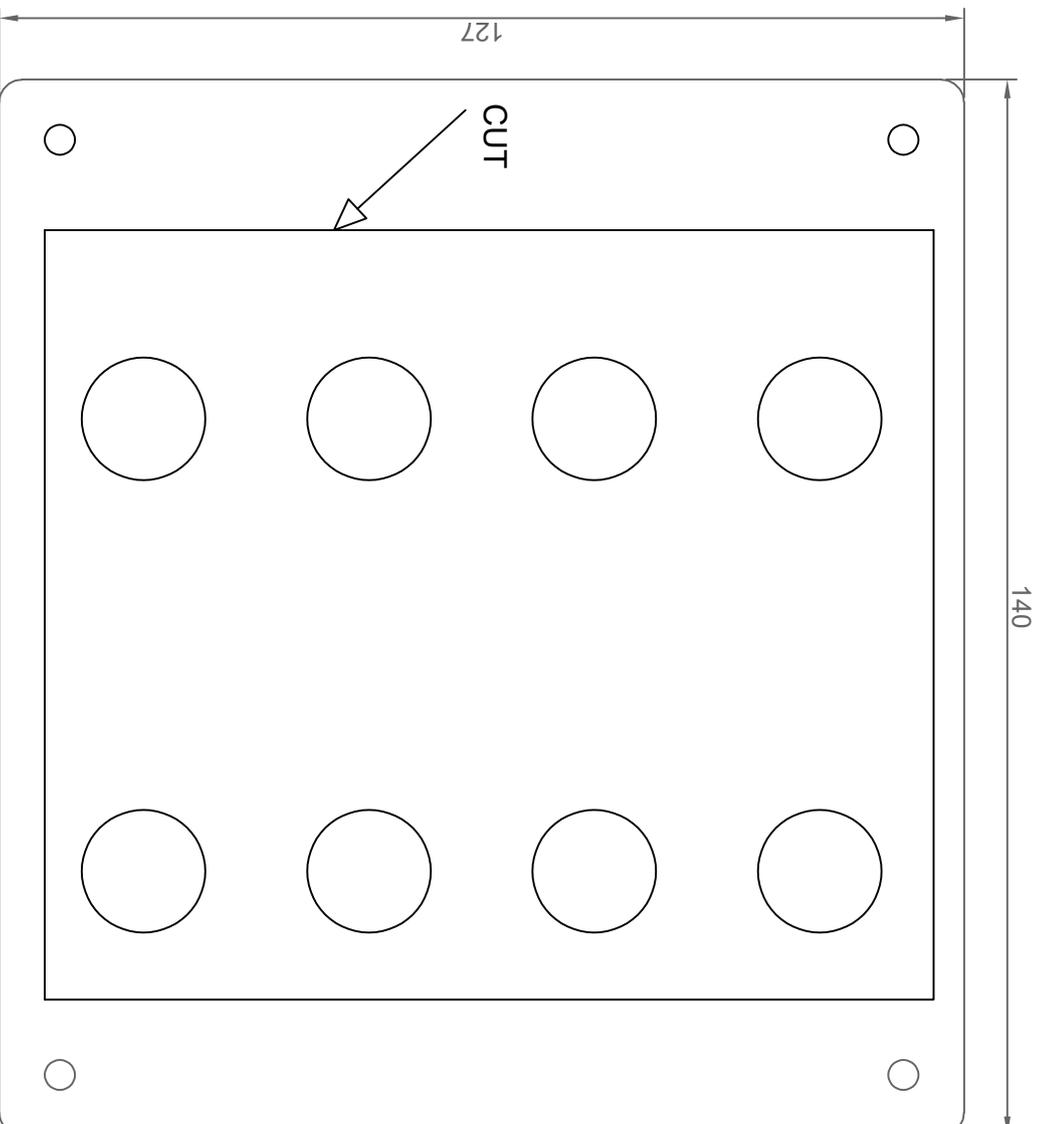
EN: Always compare this template with the switch panel, before cutting! Make sure the dimensions of the template are to scale and identical to the switch panel.
